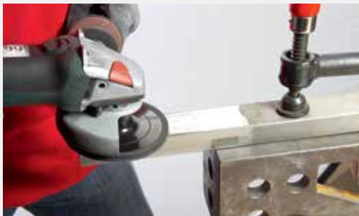
Preparation for Polishing; Metabo INOX 5" grinders, 5" 'cling fit' Pyramid sanding discs in grit range from A160 (120 grit) to A30 (600 grit) with 5" backing pad 623298000.
