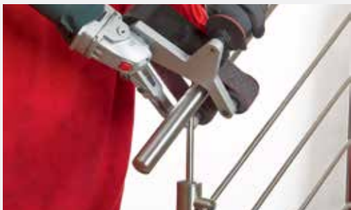
The Pipe and Tube sanders for a uniform even finish on hand rails using Pyramid sanding belts from A160 (120 grit) to A6 (2000 grit).
